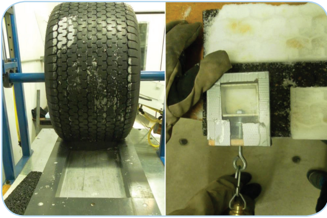
Innovative tests conducted as part of this project included compacting snow on a pavement sample, rolling a loaded tire over it 750 times and then measuring the shear force (right) necessary to plow snow from the surface.
